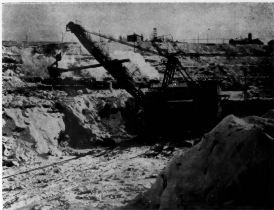
Asbestos quarry, showing large power shovel in the background. Quarry located at Eden, Vermont. (Courtesy U. S. Bureau of Mines).
